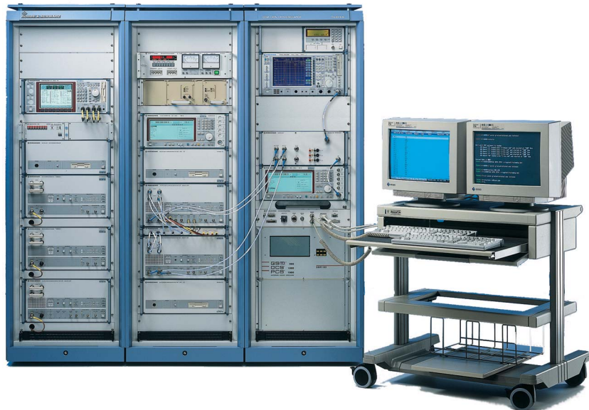
Test System R&S TS8916B with audio option for all GSM standards (photo 43211-2)
