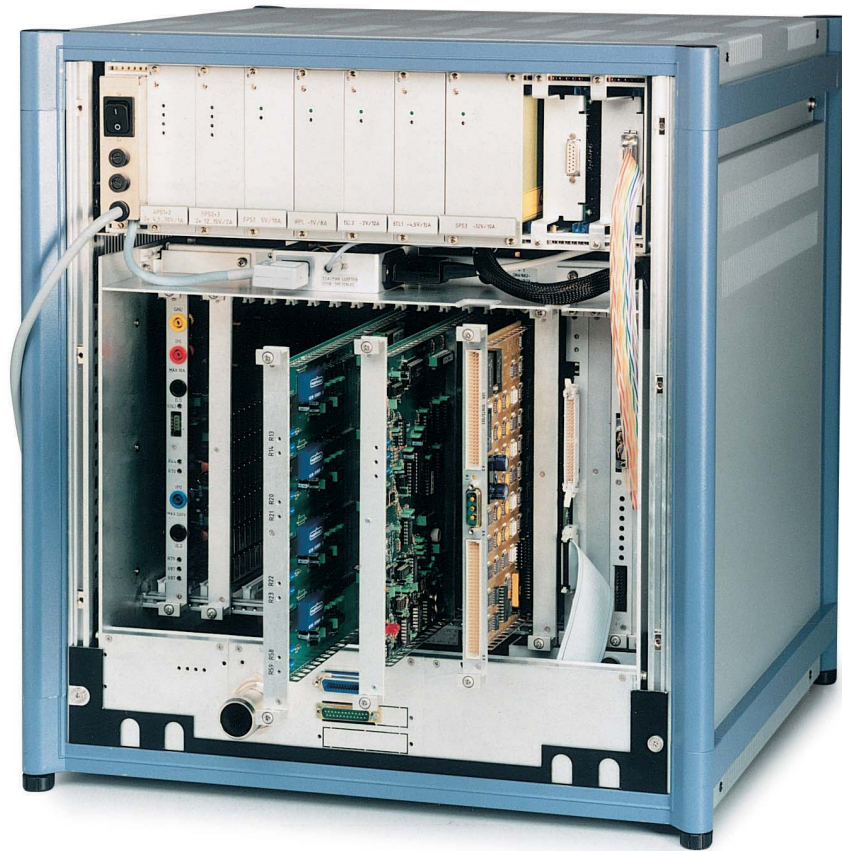
Stimulus and measurement modules are inserted into the rear of R&S TSA (photo 38860)
